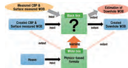
Concept of Gray box model for Downhole WOB Estimation
