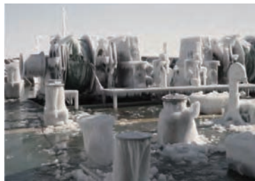
船首からの波しぶきで起きた船体着氷 Ship icing due to collision between ship bow and waves
