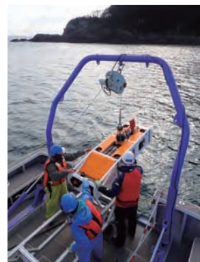
氷海探査用AUV MONACA AUV MONACA for under ice survey
