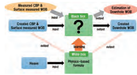
Concept of Gray box model for Downhole WOB Estimation
