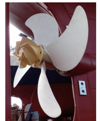
炭素繊維プラスチック製の船用プロペラ Marine propeller made of carbon fiber reinforced plastics.
