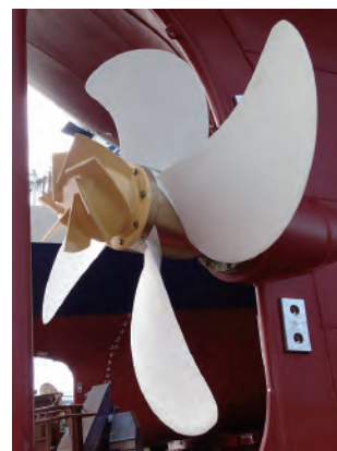
炭素繊維プラスチック製の船用プロペラ Marine propeller made of carbon fiber reinforced plastics.
