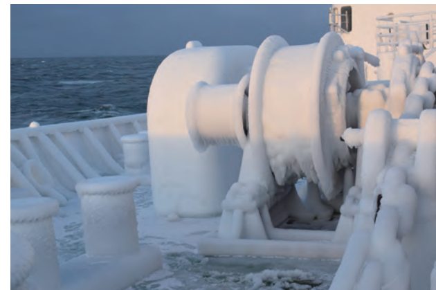
船首からの波しぶきで起きた船体着氷 Ship icing due to collision between ship bow and waves
